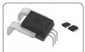
Photos of the two current sensor devices described in the text. These are sized to the same relative scale. Which one would YOU want to carry all your generator output?
